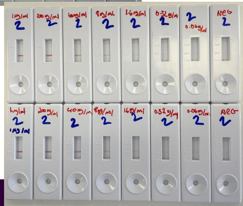
Prototype 2. mAb 32 + Colloidal Gold, mAb 8 test line
